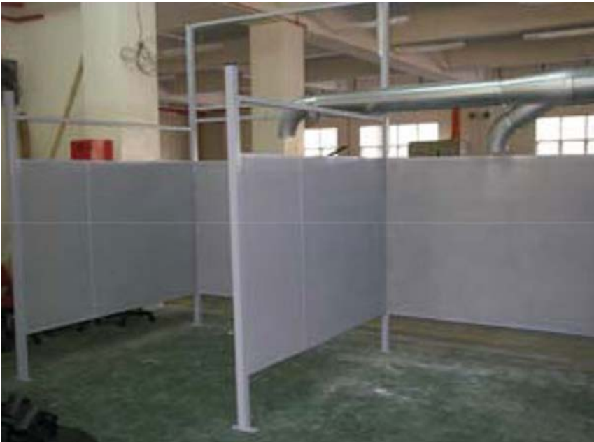
Figure 8: Welding bay partitions. Ideally the front and rear vertical support columns would extend all the way to the ceiling to provide the partitions with greater rigidity.
