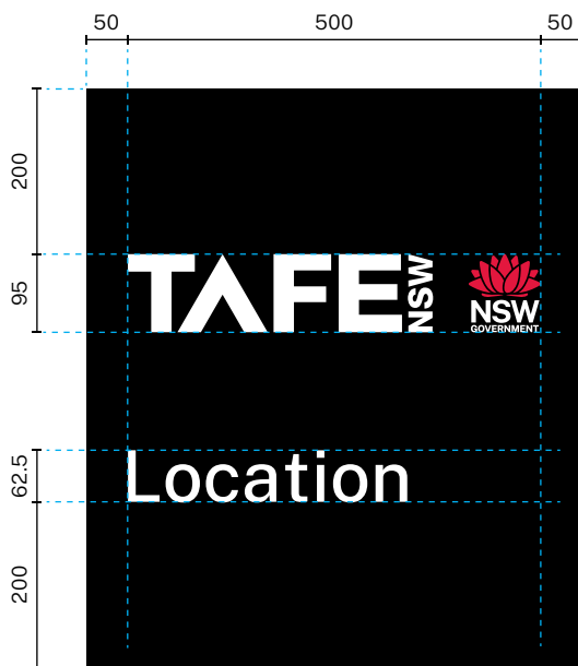
Header Panel Single line location name Scale 1:10
