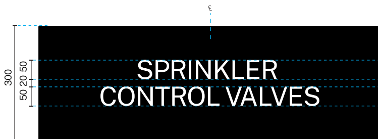
01 Door Plate Signage: 300mm Scale: 1:10
