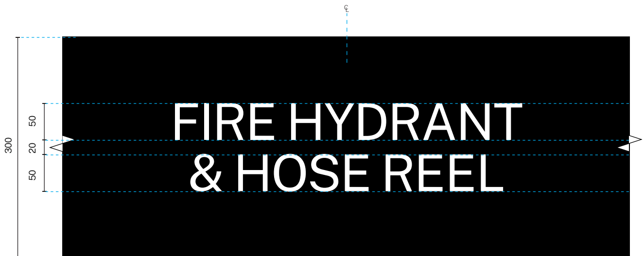
01 Door Plate Signage: 300mm Scale: 1:5
