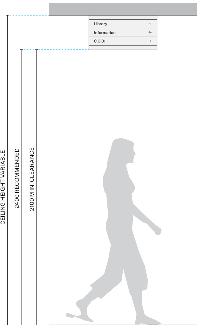
Front Elevation Scale 1:20
